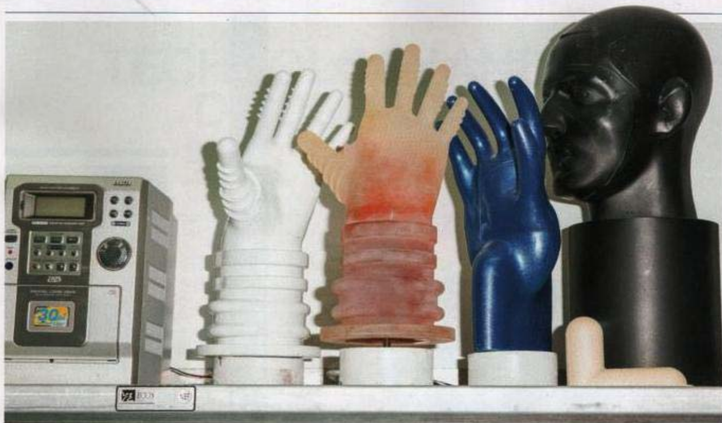
7 At engineering firm ILC Dover, which is designing a space suit for NASA, 3-D-printed glove molds are custom-made for each astronaut.
